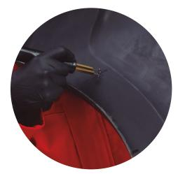
**UNIPLAST** is a hot stapler, extremely handy and easy to use. It offers a quick solution to repair and consolidate the majority of automotive plastic components in a very simple way. It has a temperature regulator which allows to heat the staple accordingly to the thickness of the plastic that needs to be repaired. The three positions of the central unit to heat the staples are:
