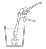
**Next,** put the cone part into the tank, and release pressure by triggering the gun for 1 minute. (Note: Special acting requires for individual tools, please refer to the instruction for us for each tools)
