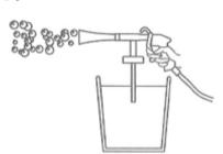
**First,** put clean water or specialized solutions into tank. Put the tube into tank, and release pressure by triggering the qun for 1~2 minutes
