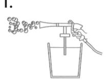
**First,** put clean water or specialized solutions into tank. Put the tube into tank, and release pressure by triggering the gun for 1~2 minutes
